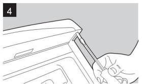
Using the flat bladed screw driver remove the pin from the top bracket. Replace it in the hinge bracket on the opposite side.
